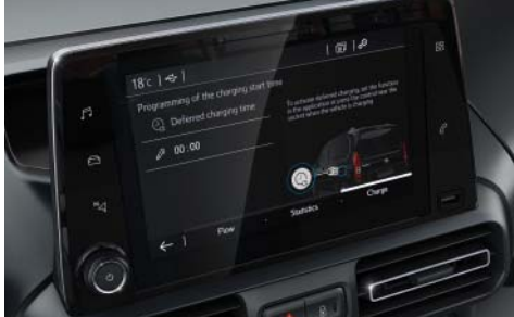
BATTERY CHARGING AND THERMAL PRE-HEATING PROGRAMMES Ensure your van's ready for you, by managing your preferred charging times and warming the cabin before the day begins.
