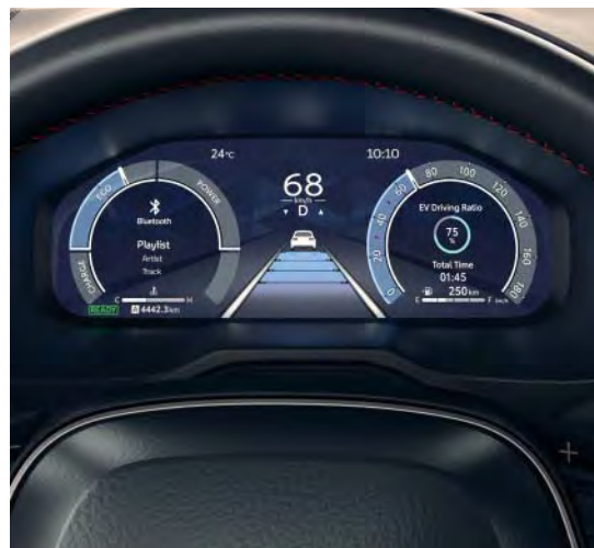
12.3" TFT combimeter A new 12.3" TFT combimeter keeps important information in your eye line while driving.
